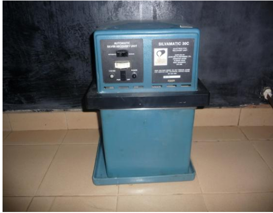
Silver Recovery Unit
